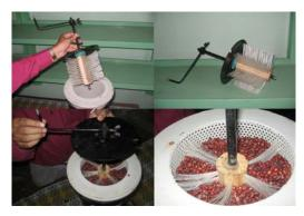
outer container and an inner perforated container with a rotating rod having fixed with plastic brushes on all sides. The seeds with eggs are to be stored in the perforated container and the rod has to rotated one full circumference clockwise and anti-clockwise for 10 minutes 3 times a day (morning, noon and afternoon). Due to the splashing action of the brush in rotating rod, the eggs get crushed and thus the damage is prevented. The treatment does not affect the germination of seeds.
