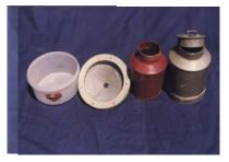
enter the perforation to reach the aerated part and while doing so, get slipped off and fall into the collection vessel through a pitfall mechanism provided in the collection vessel. In order to quickly collect the insects, as and when they emerge from grains, perforated (2 mm) rods are fixed in the inner container.
